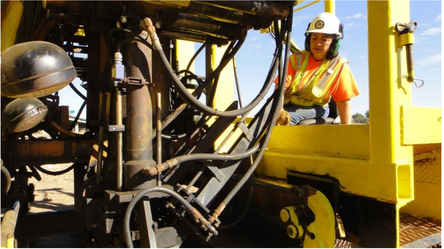
Pam loading spikes into the chutes
